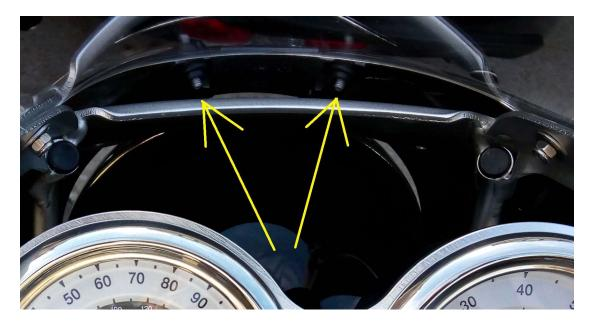
Position the screen between the metal support arms and the fairing, taking care to align the screen holes adjacent to the fairing holes.
