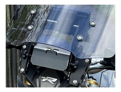
If you have selected one of our Screens, assemble the new screen screws onto the screen and hold them in place on the back-side using the rubber washers.
