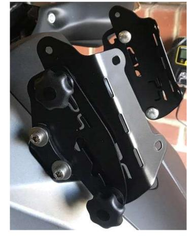
Assemble the new screen screws onto the screen and hold them in place on the back-side using the rubber washers.
