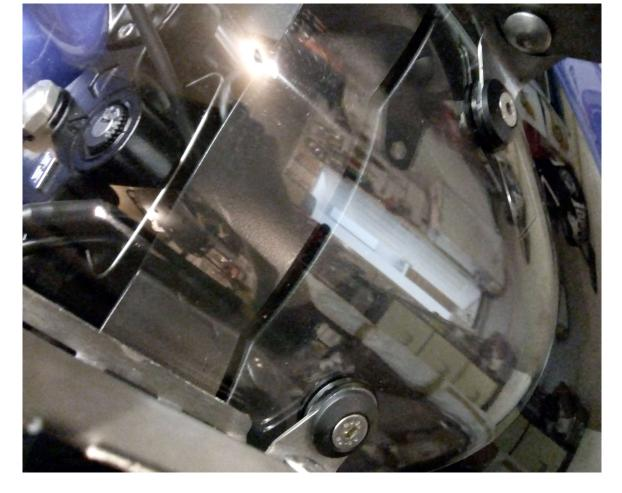
Using the fasteners provided, mount the brackets (ensuring a washer is placed between the brackets and the screen to help isolate stress and scratches) and secure underneath using the plastic washers and locknuts - do not overtighten or this may crack the screen.
