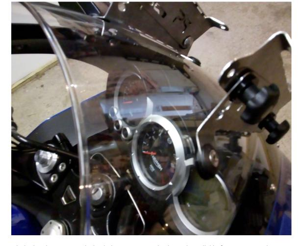
With the brackets mounted, check they are perpendicular and parallel before mounting the screen.
