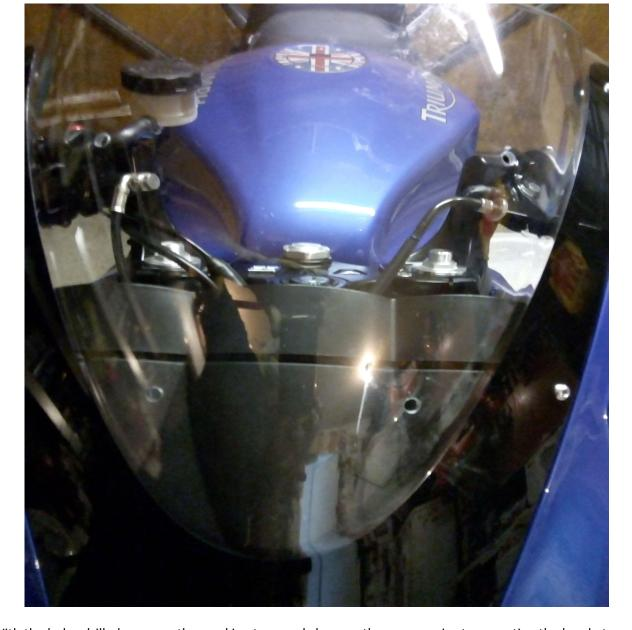
With the holes drilled, remove the masking tape and clean up the screen prior to mounting the brackets.
