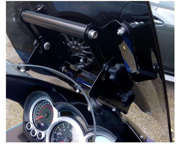
If you have selected the optional Accessory Bar, simply attach onto the existing bracket holes as shown below.
