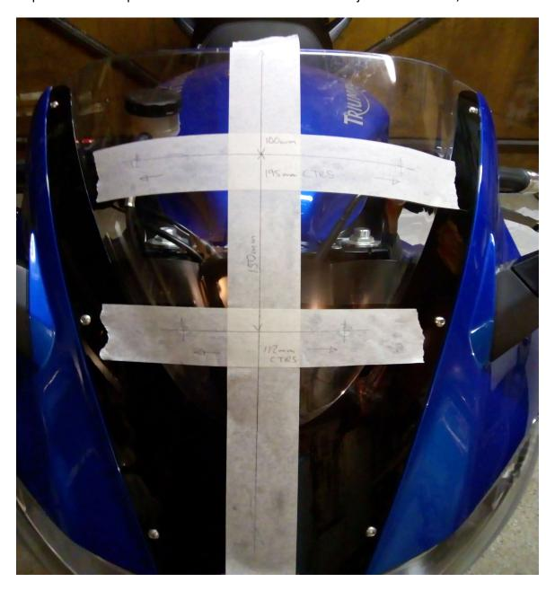
Once marked up, double check the hole positions are symmetrical and correctly spaced.
