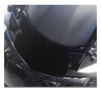
For 04-07 MY bikes, the cover plate fits on the underside of the lower bracket mounts.
