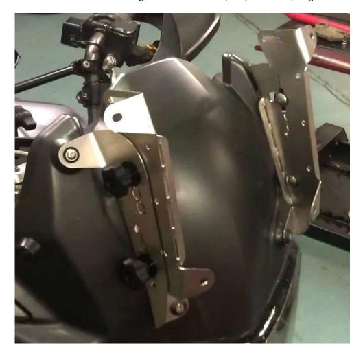
Loosely mount the bracket assemblies onto the existing screen mount holes - note: the shorter fasteners fit in the top holes and the longer ones fit in the lower rubber well-nuts.
