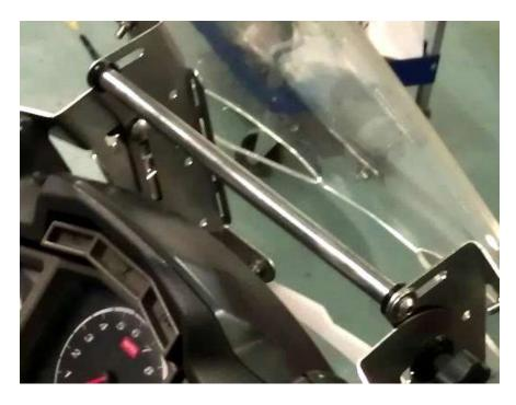
Mount the screen onto the brackets, taking care to fit a rubber washer (in each fastener location) between the screen and the metal brackets.
