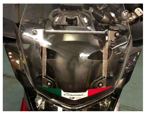
The kit also includes a set of 4 black finishing washers if your screen doesn't have recessed mounting holes, as shown above.
